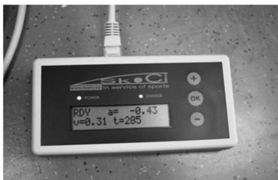
Figure 1. Device (named SkoCi) with an acceleration sensor (visible on Figure 2).
